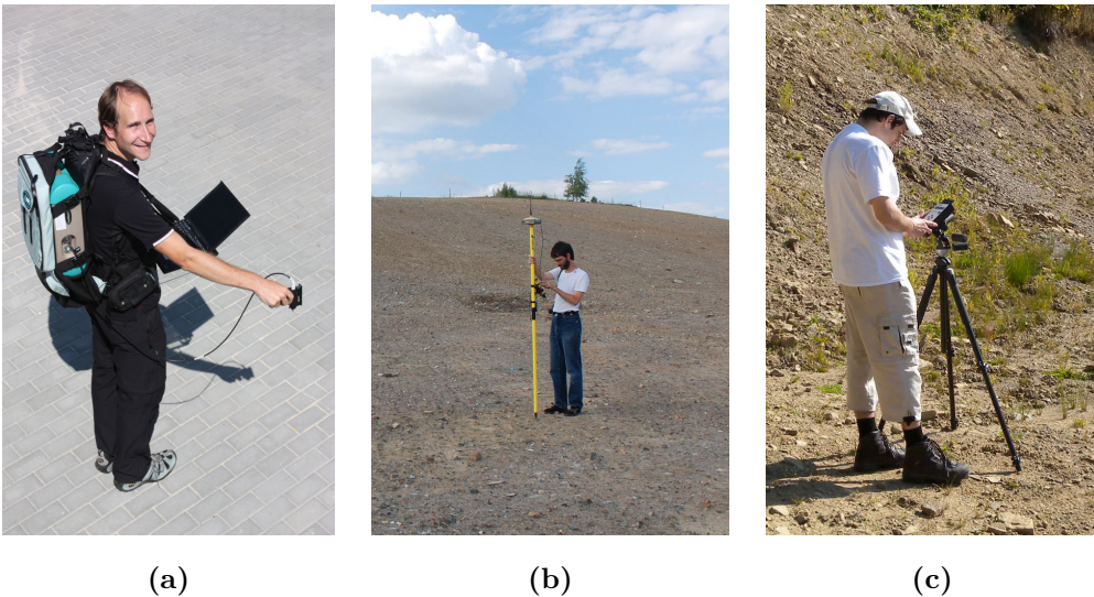
Figure 1.15 Ancillary ground measurements of (a) surface reflectance properties (ASD Field Spec-3), (b) location of geometric ground control points (TOPCON), (c) atmospheric characterisation (Microtops II).
