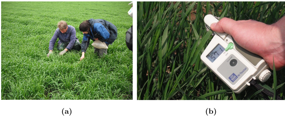
Figure 7.8 (a) Plant sampling of spring barley canopy stand at BBCH 32 and (b) chlorophyll-meter estimation of nutrition status of plants by Yara N-Tester.
